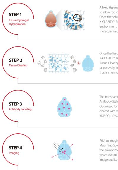
A fixed tissue sample is incubated in the X-CLARITY<sup>™</sup> Hydrogel Solution Kit to allow hydrogel monomers to diffuse uniformly throughout the sample. Once the solution has permeated the tissue, the sample is placed in the X-CLARITY<sup>™</sup> Polymerization System. Monomers polymerize in the anaerobic environment, linking the biomolecules to a hydrogel network, which preserves molecular information and structural integrity.
