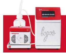
X-CLARITY<sup>™</sup> ETC Control Tower X-CLARITY<sup>™</sup> ETC Chamber X-CLARITY<sup>™</sup> Buffer Reservoir X-CLARITY<sup>™</sup> Tray 1 Container Holder for 1 Tissue Container **Tissue Containers 12 L Electrophoretic Tissue Clearing Solution**
